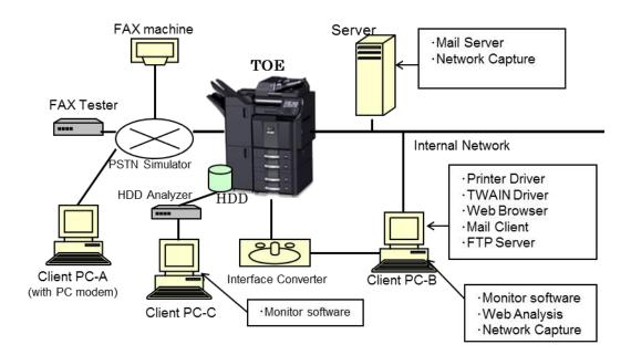
Figure 7-1 Configuration of the Developer Testing
