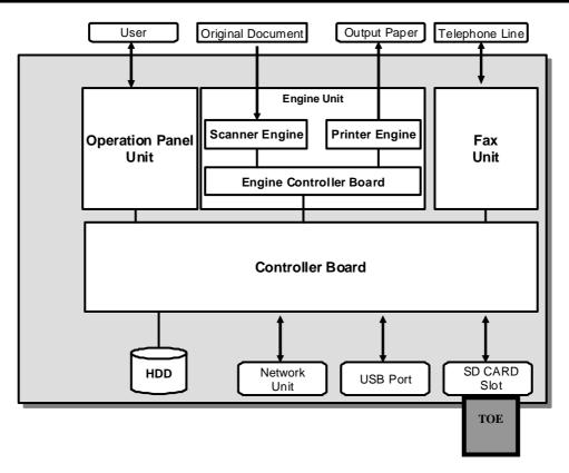
Figure 2: MFP's Hardware Configuration and TOE Positioning
