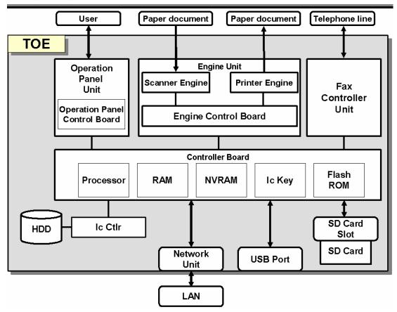
Figure 2: Hardware Configuration of the TOE
