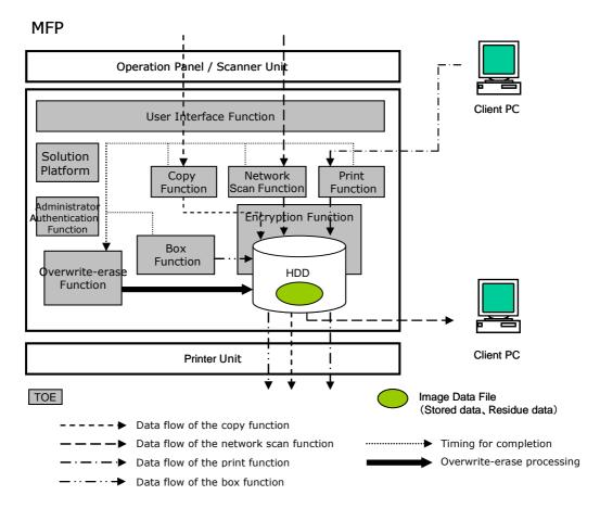
Figure 1.3 Logical Configuration of the TOE
