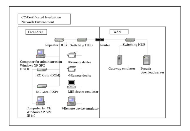
Figure 7-1 Configuration of the Developer Testing
