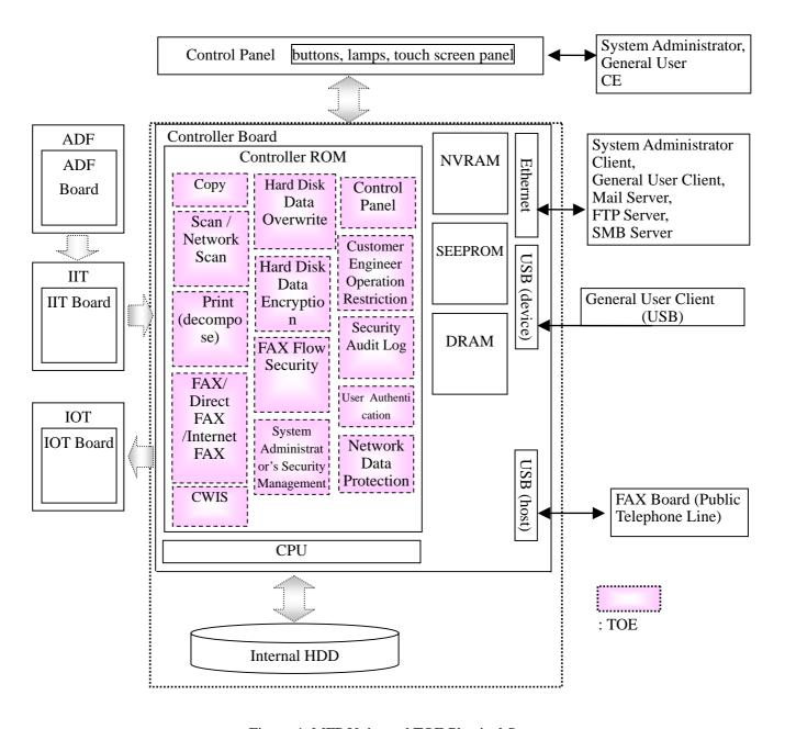
Figure 4: MFP Units and TOE Physical Scope
