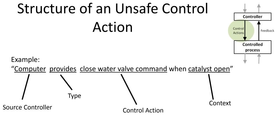
Four parts of an unsafe control action
